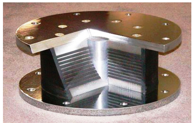
View of the interior of a lead rubber bearing (source: MCEER-07-0012)
